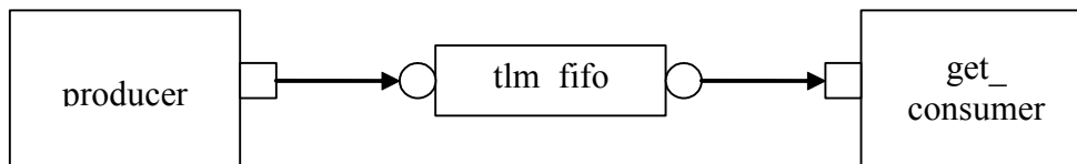
Figure 2-3 Using a tlm_fifo
